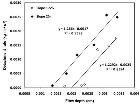
Figure 2. Relationship between detachment rate and flow depth (D) at two different slopes.
