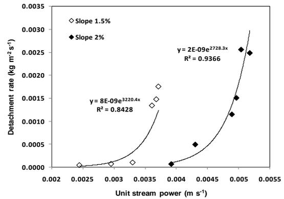
Figure 5. Detachment rate as a function of unit stream power (U=VS) at two different slopes.
