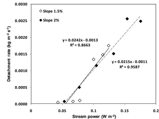
Figure 7. Relationship between detachment rate and stream power ( $\Omega = \rho g D S V$ ) at two different slopes.
