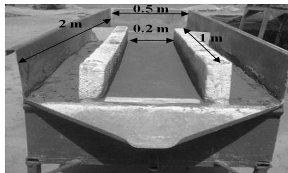
Figure 1. The applied flume for sheet flow experiment with initial ( $2 \text{ m} \times 0.5 \text{ m}$ ) and test area ( $1 \text{ m} \times 0.2 \text{ m}$ ) dimensions.
