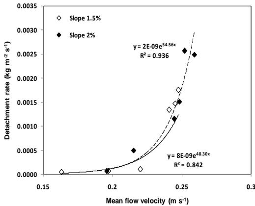
Figure 3. Detachment rate as a function of mean flow velocity (V) at two different slopes.
