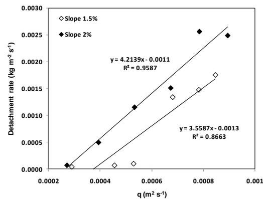
Figure 4. Relationship between detachment rate and unit flow discharge ( $q = DV$ ) at two different slopes.
