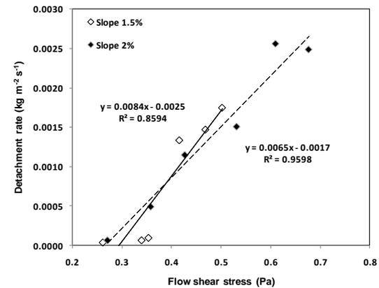
Figure 6. Relationship between detachment rate and flow shear stress ( $\tau = \rho g D S$ ) at two different slopes.
